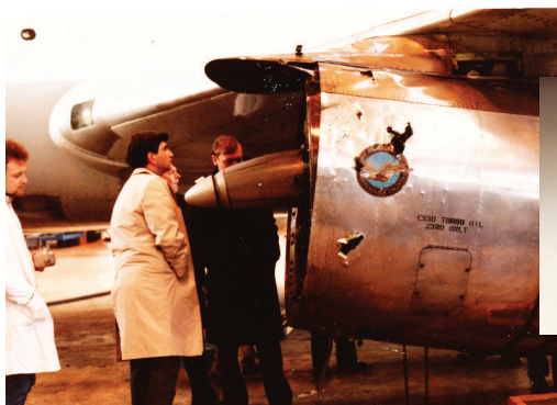
Frost (center) and others inspect damaged engine #1.
