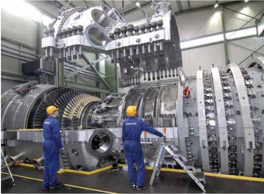
A 375-megawatt gas turbine is at the heart of 578-megawatt combined-cycle power plant in Irsching, Germany. The gas turbine alone weighs 489 tons. The combined-cycle power plant has reached a thermal efficiency of 60.75 percent, which probably makes it the most efficient heat engine ever operated. (Photograph courtesy of Siemens AG.)
